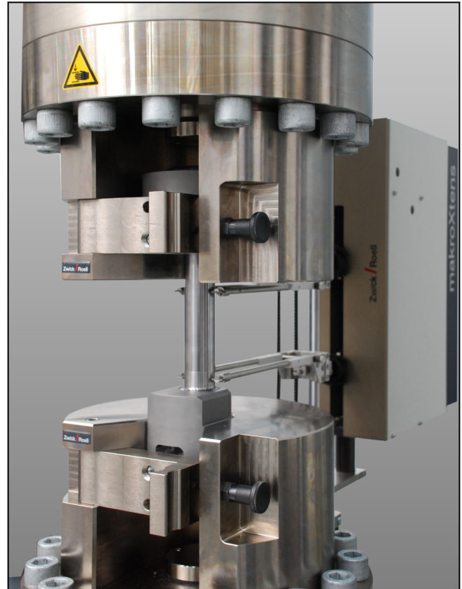
1200kN specimen grips with makroXtens extensometer on machined screw
