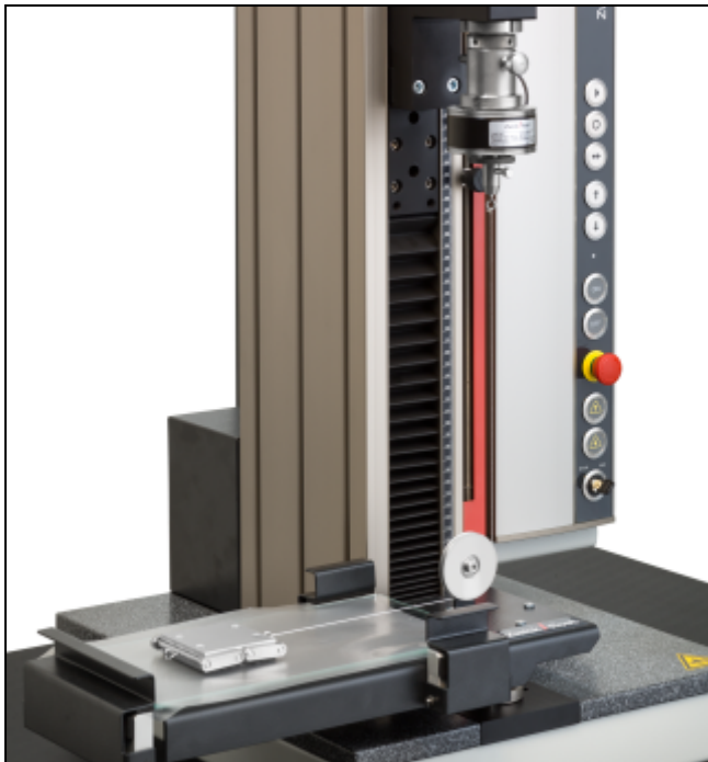
Device for testing the frictional properties of plastic films
