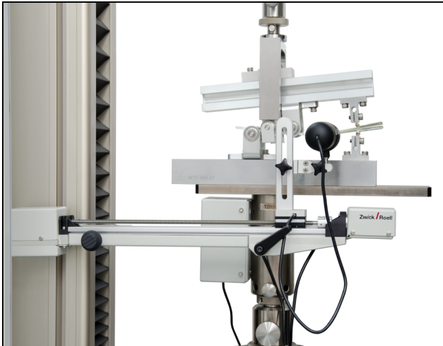
Mixed mode flexure test kit with option Video Recording
