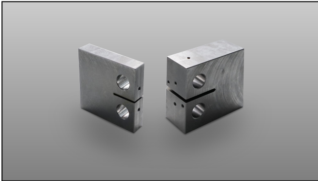
Left: CT-Specimen with W/B=4 – common geometry for ASTM E647, right: CT-Specimen with W/B=2 – common geometry for ASTM E399
